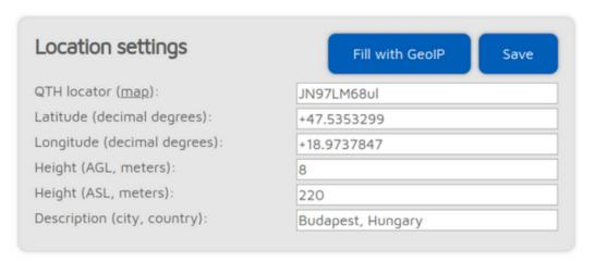
Setting location data is optional. It is used by some connectors like the <a href="Homebrew/MMDVM®">Homebrew/MMDVM®</a> to report the location of the openSPOT4 to the connector's network.
