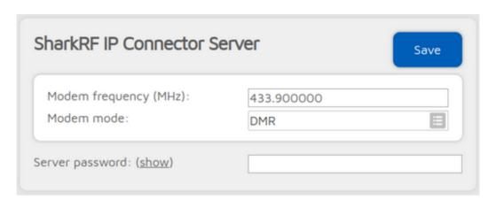
You can use this connector to accept connections from another openSPOT device. This connector only supports 1 active connection, so if you want to link more than 1 device, you can use our open source <a href="SharkRF IP Connector Protocol Server">SharkRF IP Connector Protocol Server</a>. The protocol's documentation can be found on <a href="GitHub">GitHub</a>, so you can also develop your own application for the openSPOT4.
