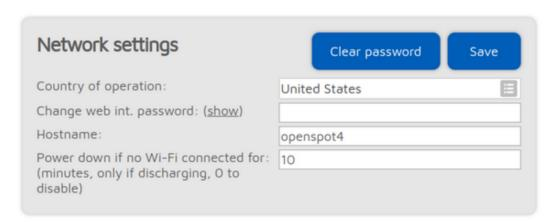
The web interface of the openSPOT4 is not password protected by default, which means anyone on the local network can open it. You can set a password by entering it in the **Change web int. password** input field. To reset the original behavior and clear the password, click on the **Clear password** button.
