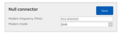
The Null connector is a special connector - as its name says - it does not connect anywhere. This is the default active connector when the openSPOT3 is unconfigured.
