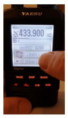
The first 5 entries will be your openSPOT3's configuration profiles. The list will contain the servers of the currently active connector. In case the currently active connector does not have a server list (ex. the Null connector), YSFReflector servers will be listed. To switch to an entry, select it using the dial and press PTT for a short time (or just tap on it in case you have a touch display).
