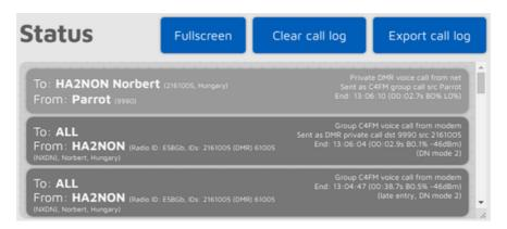
The call log displays all calls coming from the network, from the modem, or from the openSPOT3 itself (voice announcements). In modes where IDs are used as destination and source IDs (ex. DMR, NXDN®) the IDs are matched to the ID database and replaced with callsigns. You can get more information about an ID or callsign if you hover the mouse over it.
