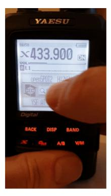
You can enter a part of the server name. All matching servers will be listed. To switch to a server, select it using the dial and press PTT for a short time (or just tap on it in case you have a touch display).
