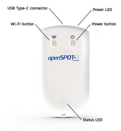
If the device is running with the factory default configuration, then there's an initialization running for about 15-20 seconds and the status LED will be blinking white:
